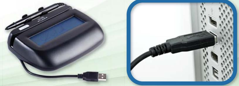
Start by inserting the USB cable into an unused USB port on your computer. No separate power connections are necessary.
